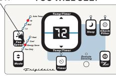
Note: In this mode, the fan will continue to run for 3 minutes after the compressor shuts off. The fan then cycles on for 2 minutes at 10 minute intervals until the room temperature is above the set temperature, at which time the unit cooling system starts again.
